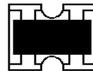
4.2  $\pm 5\%$  Tolerance of 4S02、4S03 size: the first two digits are significant figures of resistance and the third denotes number of zeros following .
