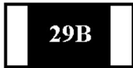
$1.96\text{K}\Omega = 196 \times 10^1\Omega = 29\text{B}$
