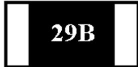
$1.96\text{K}\Omega = 196 \times 10^3 \Omega = 29\text{B}$
